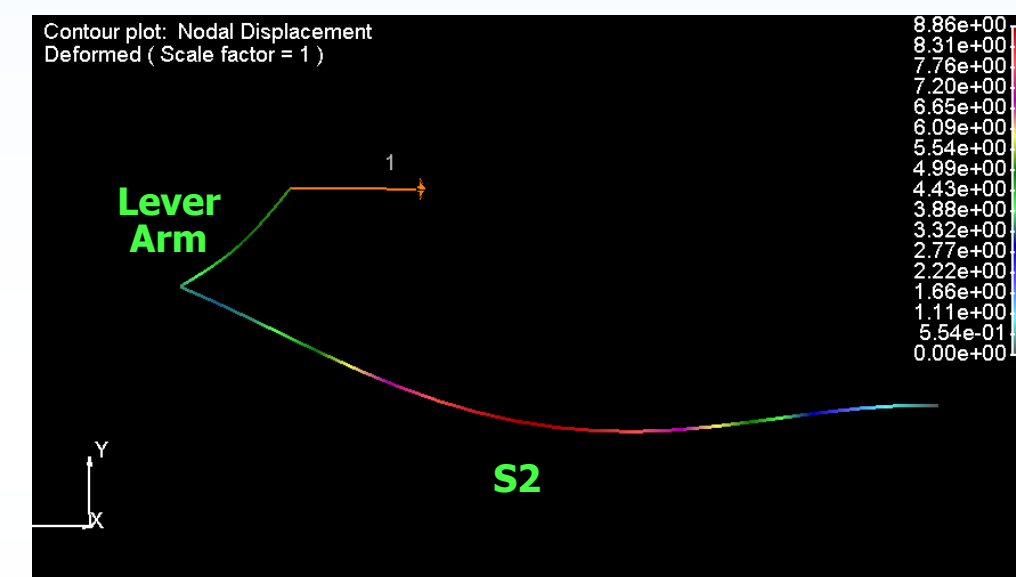
Typical crossbridge deformed configuration obtained from finite element calculations. Deformed are S2 and the lever arm. The motor domain is assumed to be rigid.
